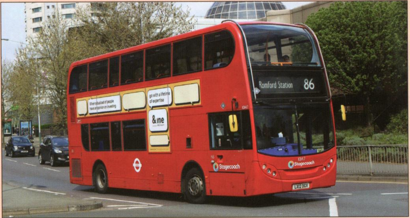
Some buses are starting to gain stickers to assist firefighters. Stagecoach Enviro400 10147 has the grey diamonds on blind box, above driver's cab and above front entrance door. For example grey is for diesel, orange for hybrid. (Richard Godfrey)
